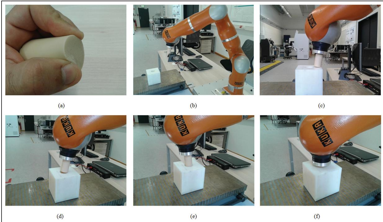
**Figure 1.** Test stand of experiment I: (a) the flexible rubber object and its deformation when it is grasped, (b) Phase 1, (c) Phase 2, (d) Phase 3, (e) Phase 4, and (f) Phase 5.
