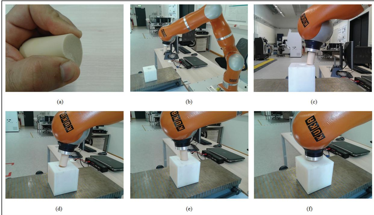
**Figure 1.** Test stand of experiment 1: (a) the flexible rubber object and its deformation when it is grasped, (b) Phase 1, (c) Phase 2, (d) Phase 3, (e) Phase 4, and (f) Phase 5.
