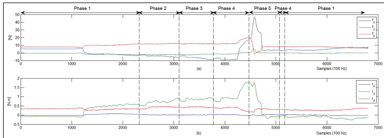
**Figure 9.** Experiment 2: training signals: (a) force signals [N] and (b) torque signals [N m].
