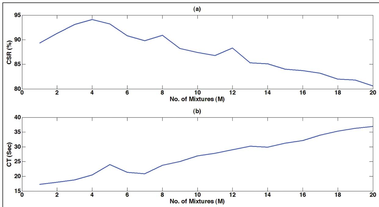
**Figure 13.** Experiment 2: DSM-GMM CS modelling scheme CSR and CT for different Gaussian components: (a) the CSR versus the number of Gaussian components ( $M$ ) and (b) the CT versus the number of Gaussian components ( $M$ ).
