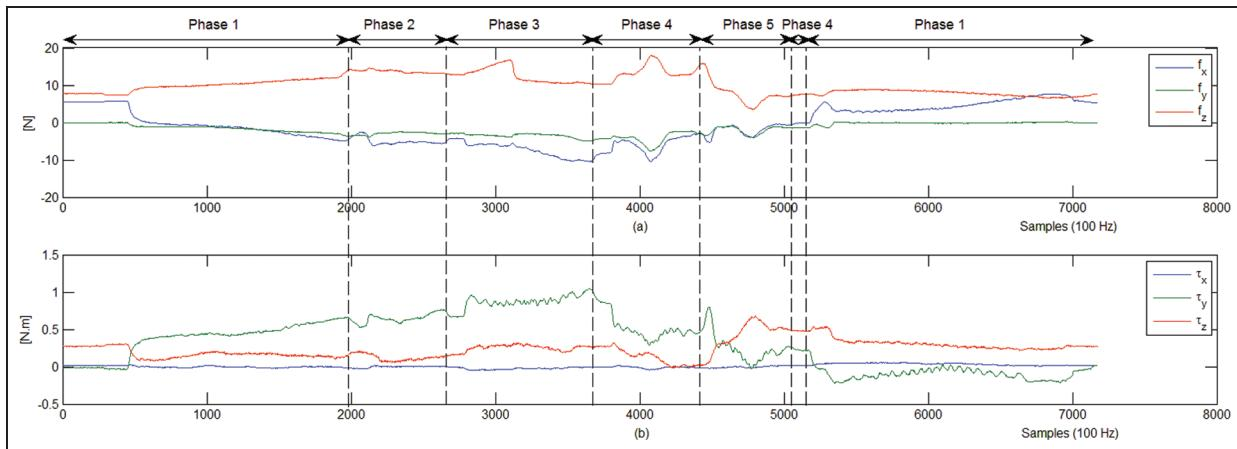
**Figure 4.** Experiment I: test signals: (a) force signals [N] and (b) torque signals [N m].
