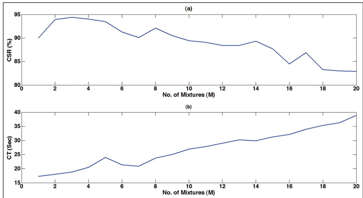
**Figure 7.** Experiment I: DSM-GMM CS modelling scheme CSR and CT for different Gaussian components: (a) the CSR versus the number of Gaussian components ( $M$ ) and (b) the CT versus the number of Gaussian components ( $M$ ).
